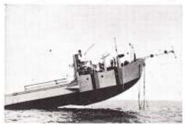
When FLIP is flooded at one end, the other end rises to form a nearly rock-solid floating platform. In 35-
